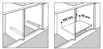
The panels of the adjacent cabinets must be made of heatresistant material. In particular, cabinets with a veneer exterior must be assembled with glues which can withstand temperatures of up to 100  $^{\circ}$ C.
